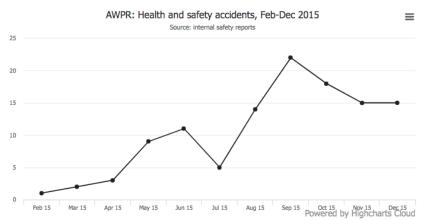
The most common types of onsite incident on the AWPR during 2015 were service strikes – when machinery hits electrical cables, telephone wires or water pipes – which accounted for a third of the total (39) incidents in those first 11 months.
